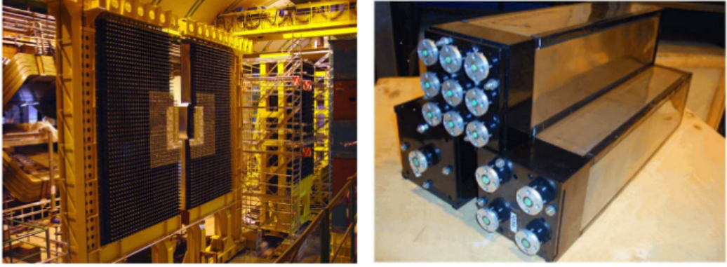
FIGURE 3.7: (Left) Downstream view of the ECAL installed (but not completely closed) with the exception of some detector elements above the beam line. (Right) Outer, middle and inner type ECAL modules.
