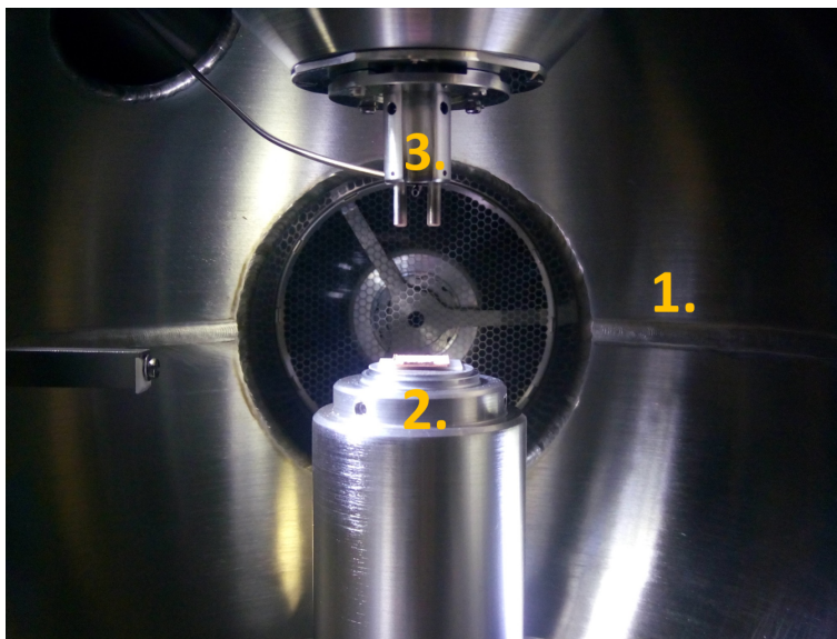
Figure 2.2. TPD system experimental set up scheme: 1. UHV chamber, 2. Heater and 3. Mass spectrometer
