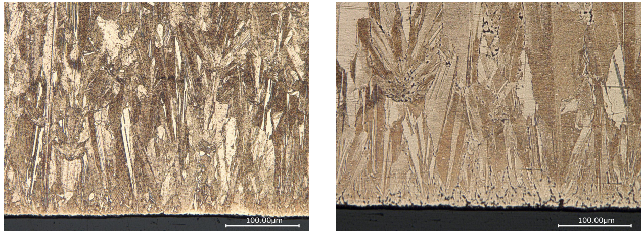
Figure 5.25. Optical microscope images after etching the cross section of samples from the matt bath. 40 A dm -2 20 ms pulse ON (a) and 40 A dm -2 80 ms pulse ON (b)
