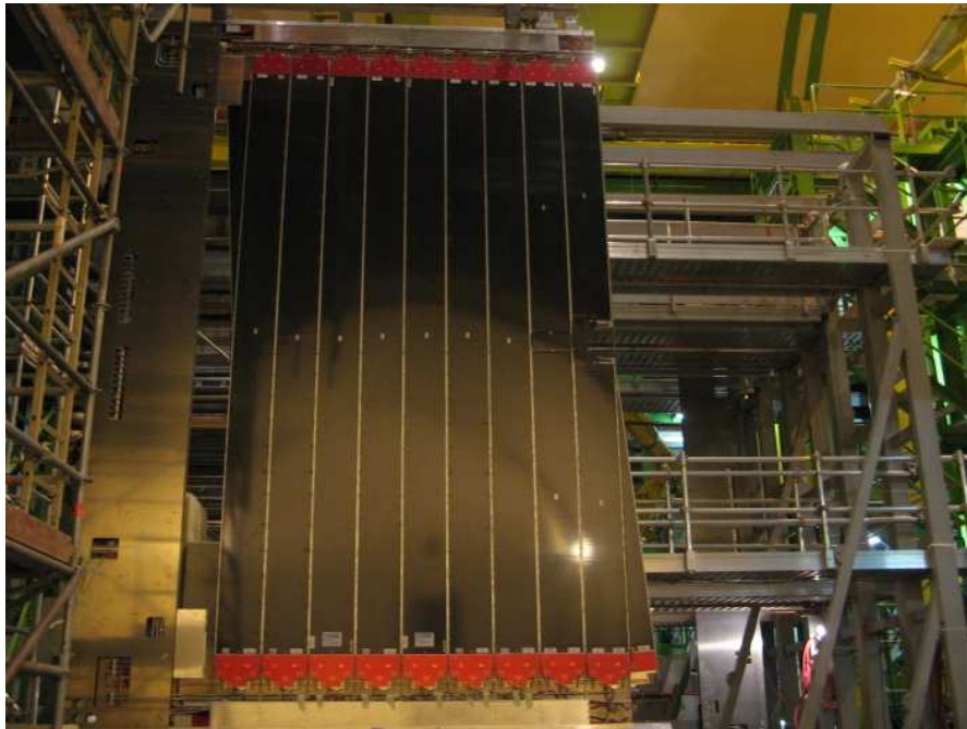
Figure 2.4: C-frame equipped with modules and Front End electronics. The frame is in mid air, being transferred from an assembly structure (C-cage) to its position in the LHCb detector.
