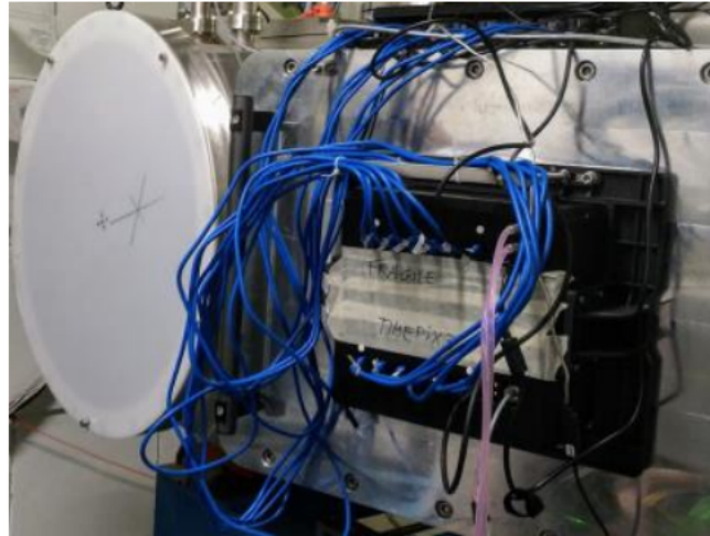
Figure 13.12: Photo of PADME's Timepix3 beam monitoring device.
