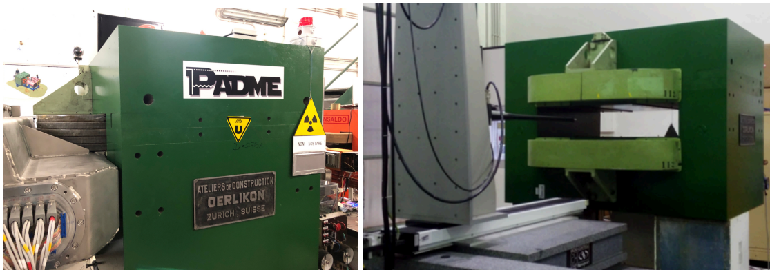
Figure 13.8: PADME’s dipole magnet: back (left) and front (right). The magnet has a 0.55 T field and a 23 cm vertical aperture.
