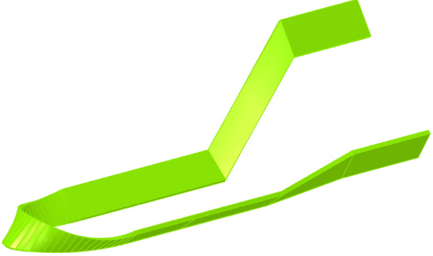
Figure 5.24: End side of one of the cables of the TCT model in Opera 3D
