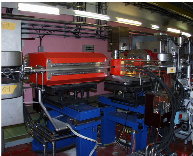
Figure 2.13: On the left, a DC septum installed in the CERN PS that is identical to the SM1 septum used in the AA
