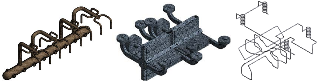
Figure 28. Left: VR (shell). Middle: SAS (solid). Right: SAS+CL cooling channel (line).
