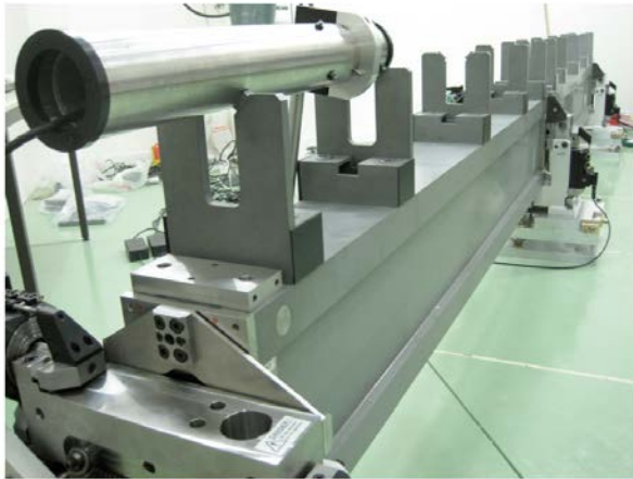
Figure 15. MB girder and V-shaped supports for CLIC prototype module 0.
