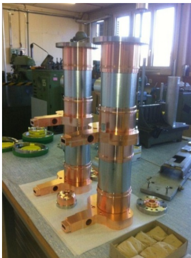
Figure 6. The octants (left) and an assembled PETS unit (right).
