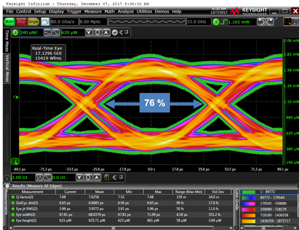
Figure 3.10 – Oscilloscope eye diagram of one MSP MGT output running at 11.2 Gb/s
