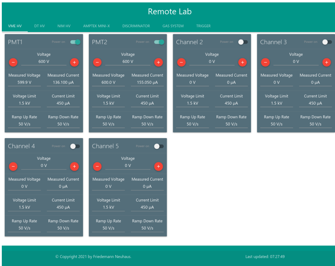
Figure B.4: Screenshot of the web interface for the lab control system. Each device has its own tab selectable on the top. The screenshot shows the tab for a high voltage power supply with two channels switched on.
