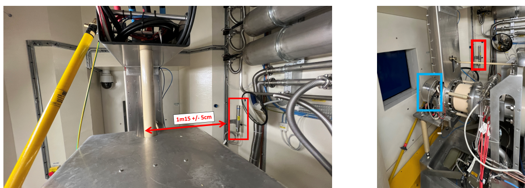
Figure 3.2: Dose rate probe (red) with respect to the MEDICIS target (blue).
