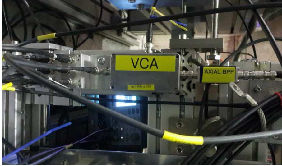
Figure 5.6: Active feedback cooling system attached to the apparatus
