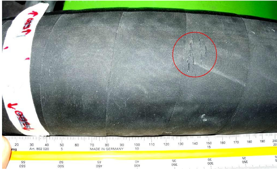
Figure 6.5: Photograph of crack-area 32 in Point 6L during the monitoring 2010. Angular misalignment and offset of reference object to crack-area are clearly visible.
