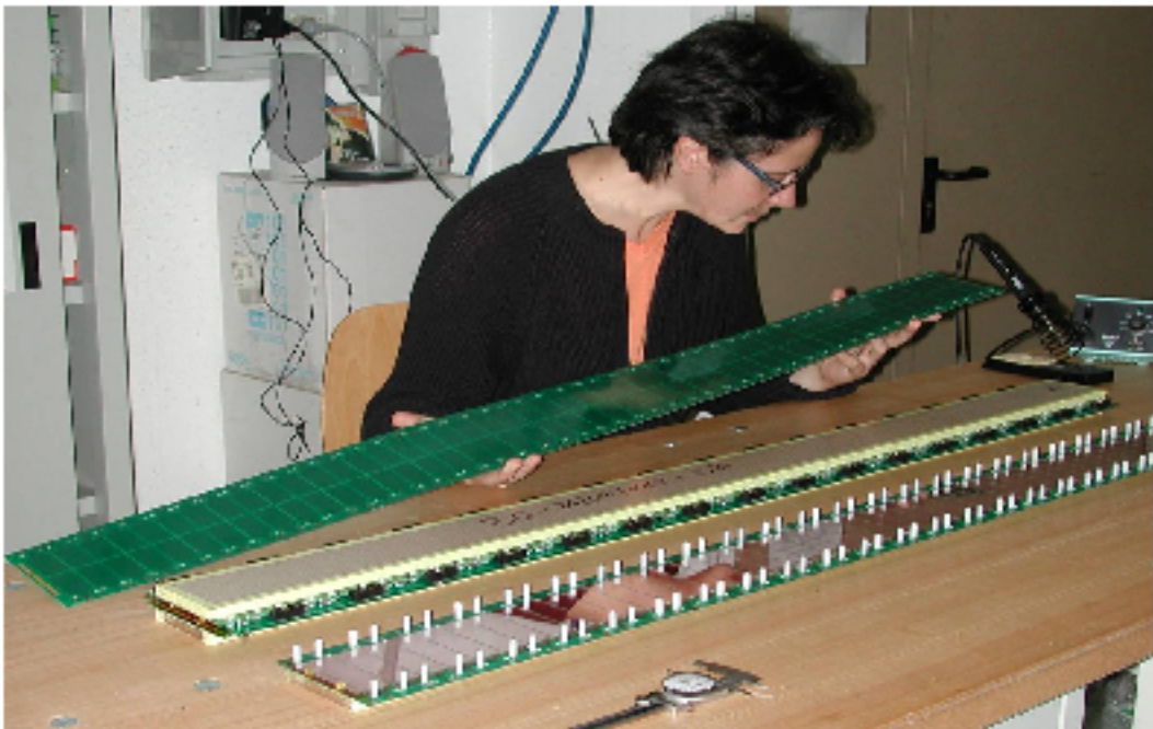
Figure 2.6: Photograph of a TOF MRPC during the assembly phase.
