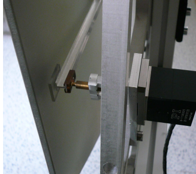
Figure 5.36: Laboratory setup, the mirror rear side: the piezo actuator replaces one of the micrometric screws.
