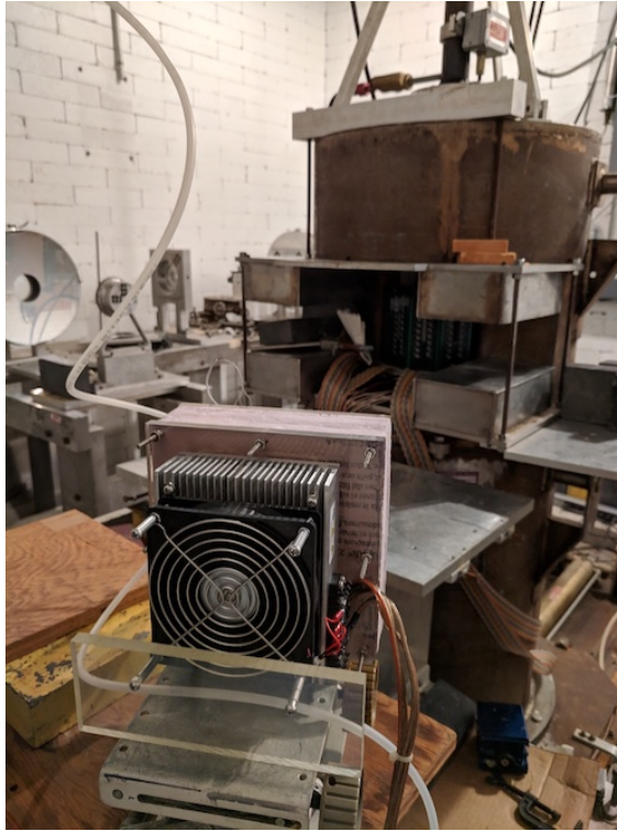
Figure 9.29: The AMACv2 coldbox located in front of the Co-60 source.
