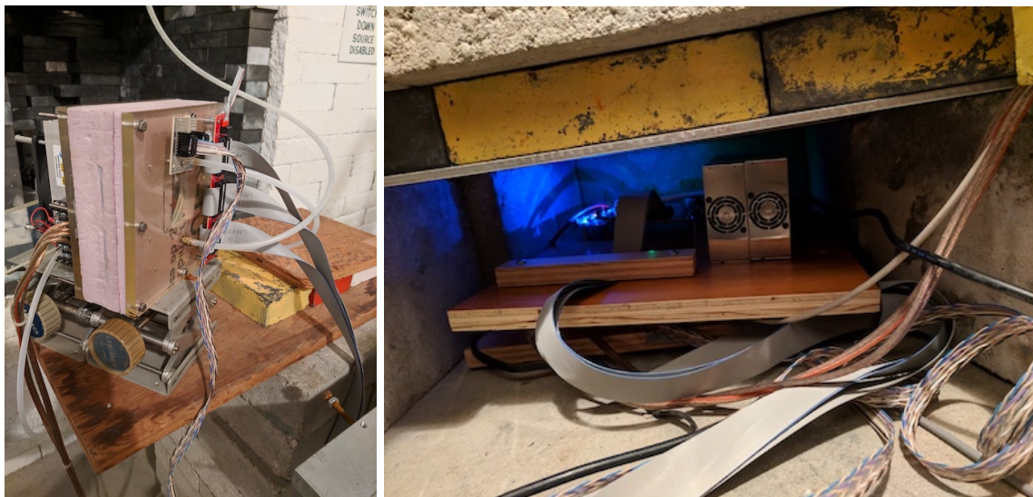
Figure 9.28: Left: Coldbox surrounding the AMACv2 chip and carrier board. The pink foam was used to prevent leakage of the nitrogen gas, while the metal device on the left-hand side of the picture is the peltier and a fan necessary for the cooling. Plastic tubes can be seen on the right-hand side of the picture, which were used to provide the nitrogen flow (one tube for nitrogen coming into the coldbox, one for nitrogen leaving the coldbox). Various cables can be seen which were used for the carrier board to test/control board communication as well as to control the peltier and to monitor the temperature and humidity in the box. The humidity sensor is not radiation-hard, and thus was only used to measure the humidity before the irradiation began. Right: The inside of the lead hut used during the AMACv2 irradiation. Two wood boards containing various components were located in the hut. The bottom board was used for the temperature control and humidity monitoring, while the top board contained the AMACv2 test/control board as well as its power supplies.
