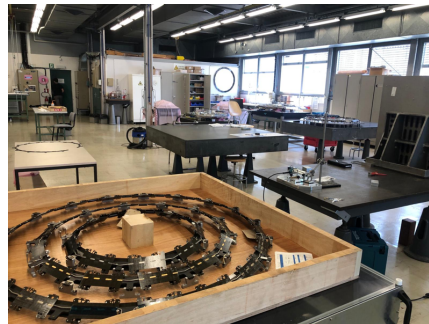
Figure 47- Rings L1, L2, and L3 ready for shipment to the Lyon Cold Room from the production building for thermal quality control.
