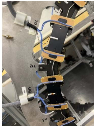
Figure 58 - Picture representing the 3 screws (labelled with red numbers) to tighten in order to place the dummy module on the ring (left) and cables secured to the setup using clips (right) to prevent loose wires.
