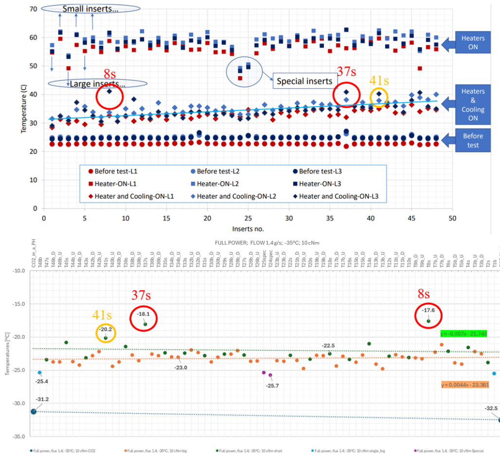
Figure 122- Comparative analysis of the TQC test results conducted in Pakistan at NCP [40] (above) and those conducted at CERN (below). The same inserts identified as anomalous in both tests are highlighted in red and yellow.
