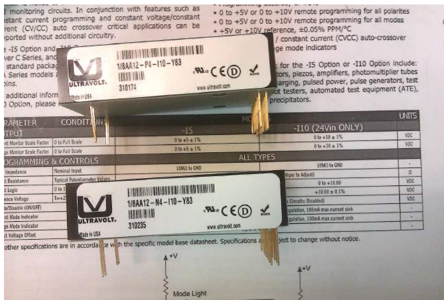
Figure 2.7: photo of two UltraVolt brand new prototypes (-Y83), a positive output 1/8AA12-P4-I10 and a negative output 1/8AA12-N4-I10 .
