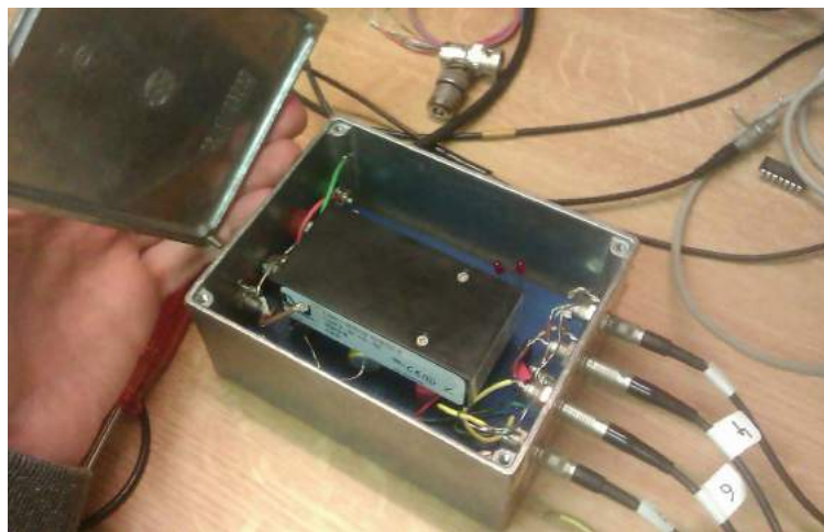
Figure 2.10: metal box for the new power supply with two leds indicating if the block is working as current or voltage generator.
