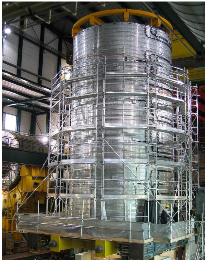
Figure 2.12: The CMS superconducting solenoid completely assembled in its vertical position.
