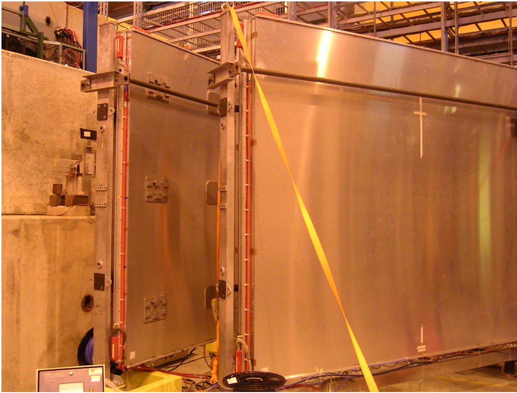
Figure 5.2: Photo of the Drift Tube Chambers experimental setup. In the photo, MB2 is partially rotated around a central vertical axis.
