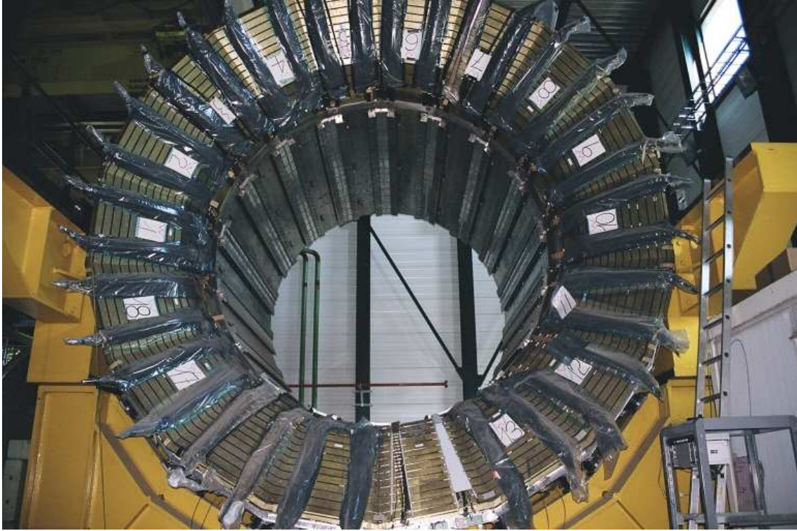
Figure 2.20: Photo of the Hadron Calorimeter Barrel (HB) in the test-bench, ready for its calibration with cosmics and a radioactive source.
