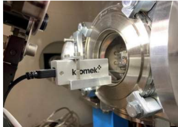
(b) Picture of the GR1 detector mounted in front of the collection box. Ref. [35].
