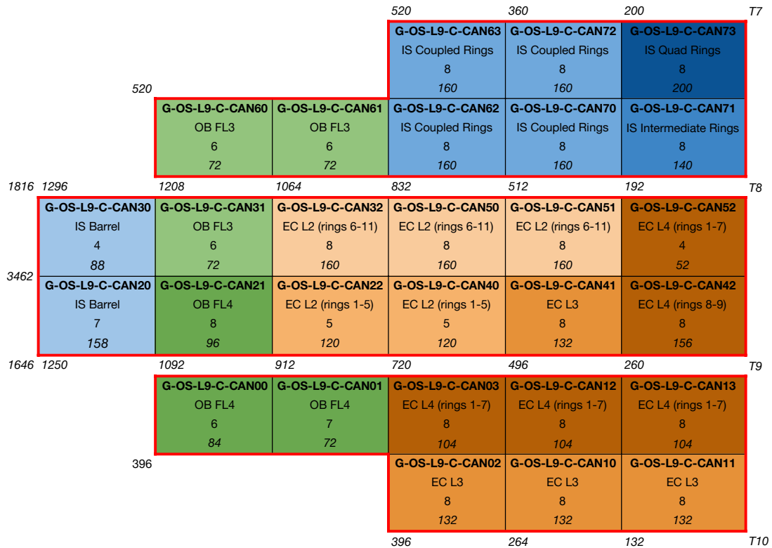
Figure C.6: Optobox distribution in the C side sector 9 Optopanel (DFT c4-5). Each box represents an Optobox, its background colour is to distinguish the different layers. The Optobox ID is bold and the layer name is given below. The first number in each box is the amount of Optoboards and the italic number the amount of Twinax cables ending at that Optobox. The thicker, coloured border indicates the source of powering cavern.
