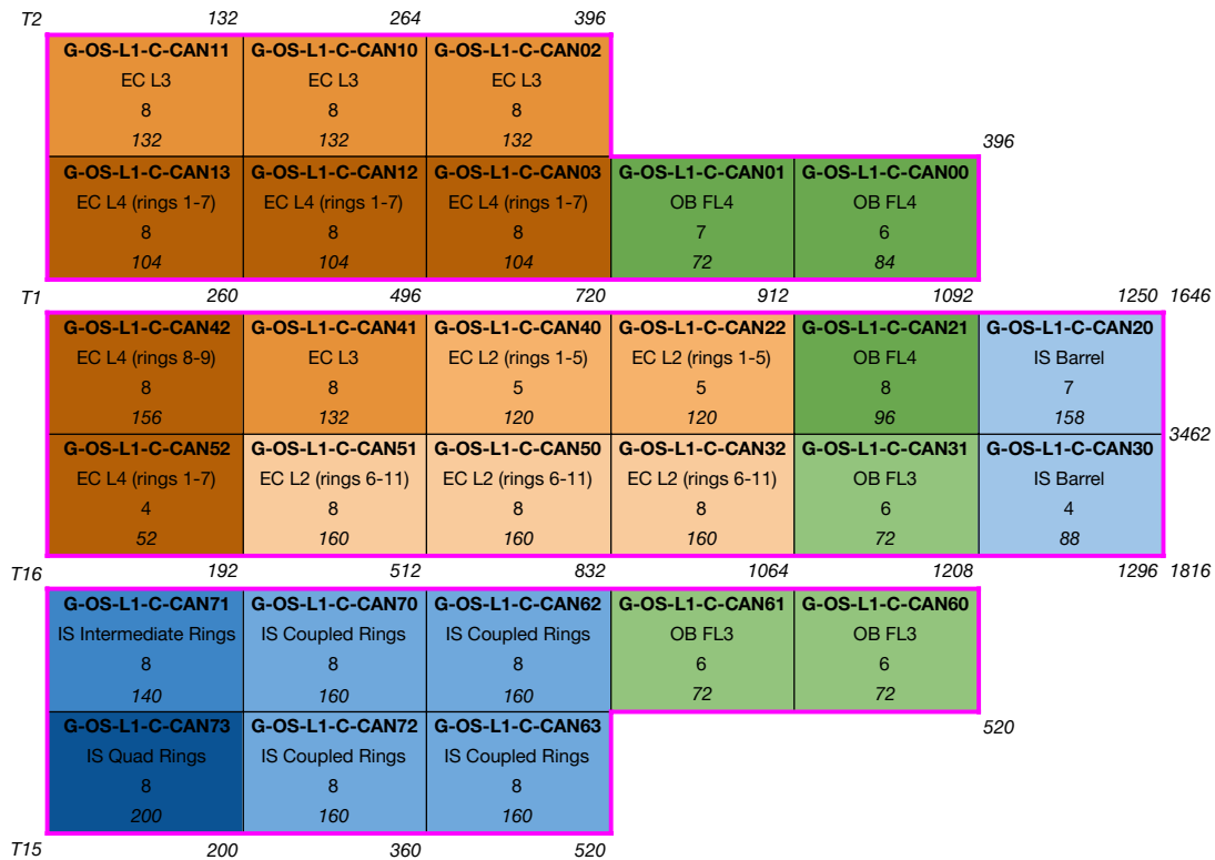
Figure C.4: Optobox distribution in the C side sector 1 Optopanel (DFT c1-8). Each box represents an Optobox, its background colour is to distinguish the different layers. The Optobox ID is bold and the layer name is given below. The first number in each box is the amount of Optoboards and the italic number the amount of Twinax cables ending at that Optobox. The thicker, coloured border indicates the source of powering cavern.
