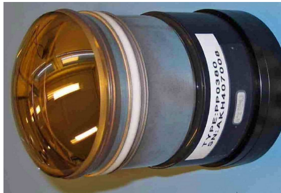
Figure 2.1. A pixel HPD used in the RICH detectors of LHCb [5].
