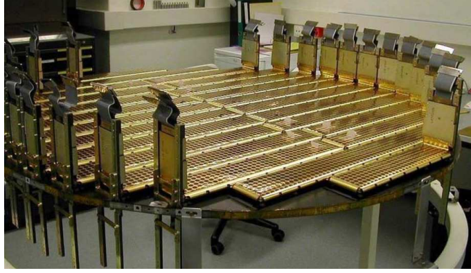
Figure 2.3: Tracker Plane equipped with ladders
