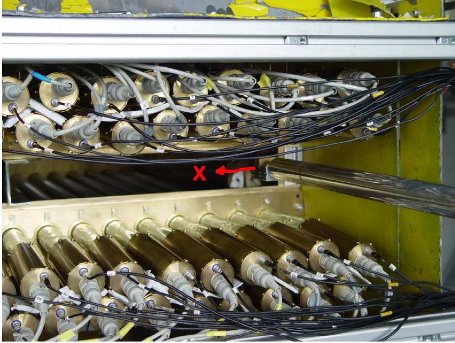
Figure 4.6: Detail view of the fully assembled component test with the strong sources removed. The box is opened to allow for a pulse height scan along the tubes with the weak source.
