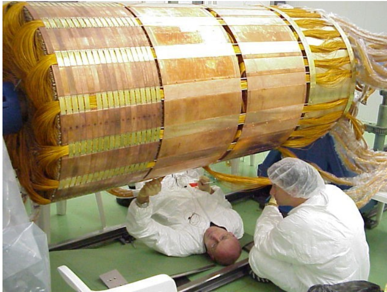
Figure 3.13: Picture of the assembly of the FCAL [86].
